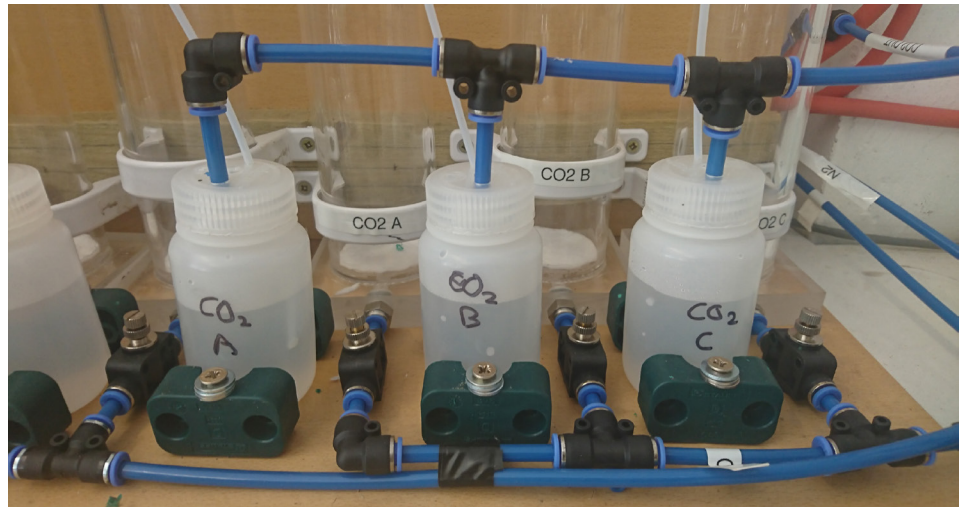
Customized upflow testing to evaluate carbonation of ultramafic tailings.
